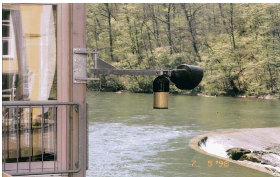
Figure 5.2: Typical Ultrasonic - in air (look down) water level sensor
